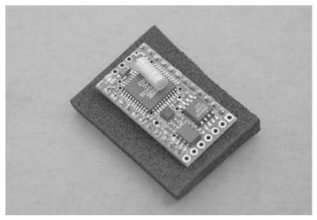
FIGURE 32.1 The BasicX-24 consists of surface-mount integrated circuits on a small circuit board. The BX-24 circuit board has the same dimensions as a standard 24-pin IC.
