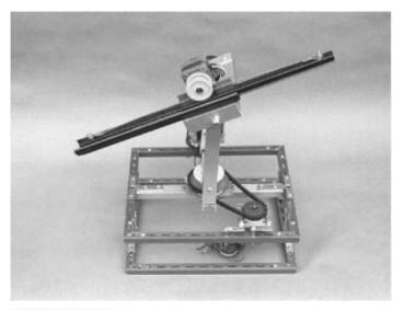
FIGURE 26.13 The finished polar coordinate arm.
