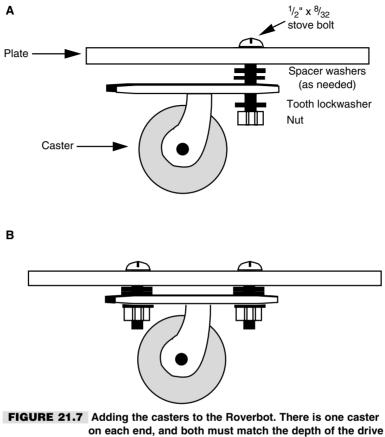
on each end, and both must match the depth of the drive wheels (a little short is even better). *a.* Hardware detail; *b.* Caster mounted on mending plate.
