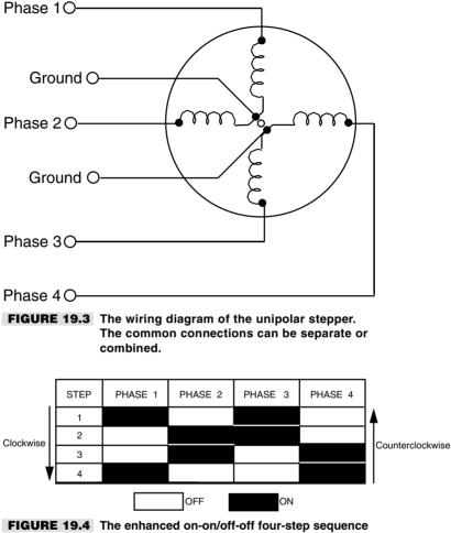
of a unipolar stepper motor.
