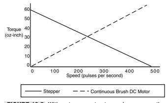
FIGURE 19.5 With a stepper motor, torque increases as the speed of the motor is reduced.
